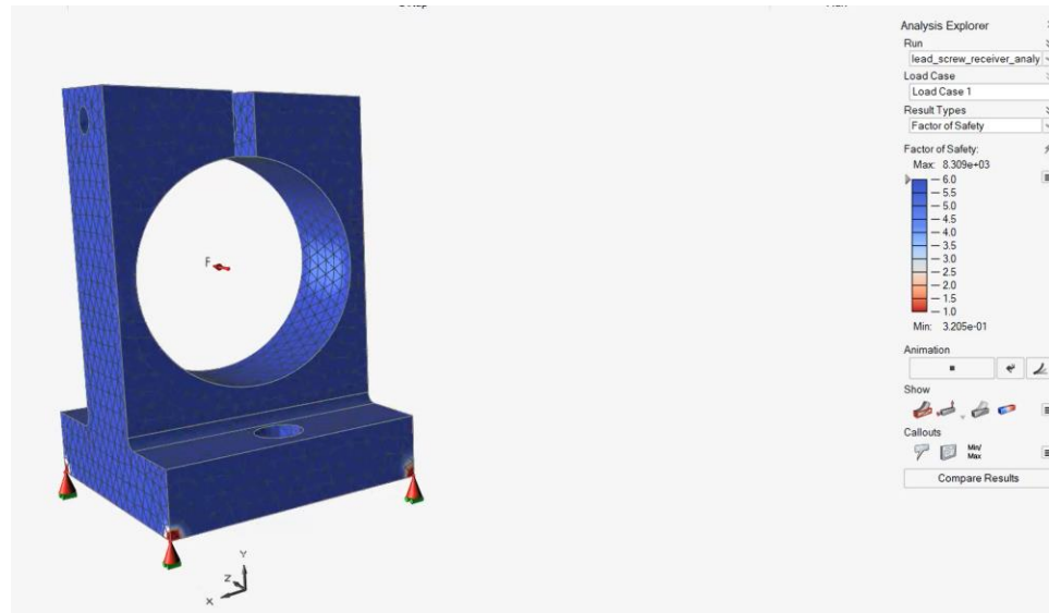
Figure I.2.3: Inspire FEA Analysis of Lead Screw Receiver Using Factor of Safety
