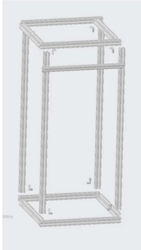
Figure H.1.7 Exploded View of the Superstructure Assembly
